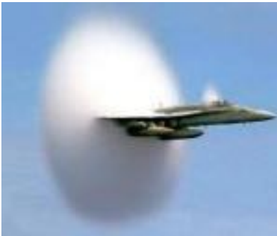
As in figure aa, this plane shows a shock wave. The sudden decompression of the air causes water droplets to condense, forming a cloud.
