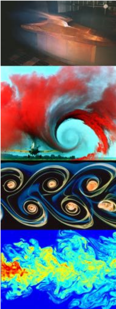
q / Fluid friction depends on the fluid's pattern of flow, so it is more complicated than friction between solids, and there are no simple, universally applicable formulas to calculate it. From top to bottom: supersonic wind tunnel, vortex created by a crop duster, series of vortices created by a single object, turbulence.
