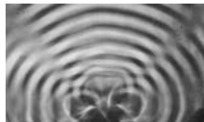
A pretty good simulation of the single-slit pattern of figure v, made by using three motors to produce overlapping ripples from three neighboring points in the water.
