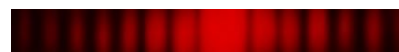
Single-slit diffraction of red light. Note the double width of the central maximum.
