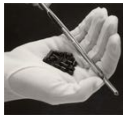
These pellets of uranium fuel will be inserted into the metal fuel rod and used in a nuclear reactor. The pellets emit alpha and beta radiation, which the gloves are thick enough to stop.
