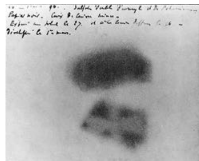
Becquerel's photographic plate. In the exposure at the bottom of the image, he has found that he could absorb the radiations, casting the shadow of a Maltese cross that was placed between the plate and the uranium salts.
