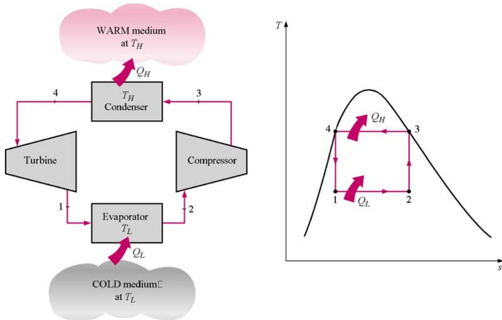
The standard of comparison for refrigeration cycles is the *reversed Carnot cycle*. A refrigerator or heat pump that operates on the reversed Carnot cycle is called a *Carnot refrigerator* or a *Carnot heat pump*, and their COPs are
