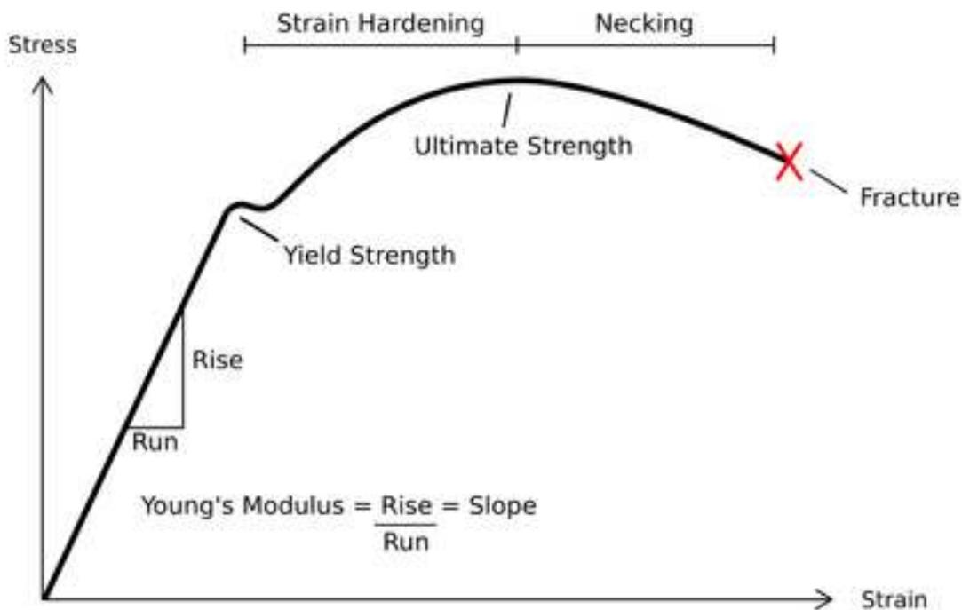
Figure 1 Typical Stress-Strain Diagram for a Ductile Material. Figure contributed by user Brakeydown under a [Creative Commons Attribution-Share Alike 3.0 Unported](#) license. The original version can be found at [this link](#).
