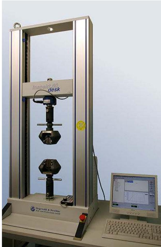
Figure 2 Photograph of a universal test device. Contributor: Rainer Knäpper. License: artlibre. [Downloaded from Wikimedia Commons.](#)
