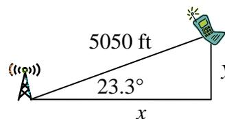
Note that if you didn't know if you were north of both towers, our calculations would have given two possible locations, one north of the highway and one south. To resolve this ambiguity in real world situations, locating a position using triangulation requires a signal from a third tower.
