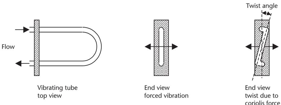
**Figure 9.16** Mass flow meter using coriolis force.
