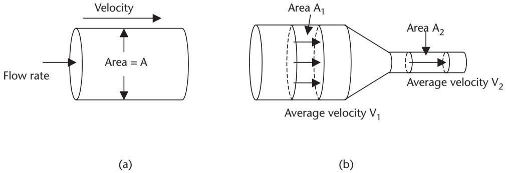
**Figure 9.3** Flow diagram for use in the continuity equation with (a) constant area, and (b) differential areas.
