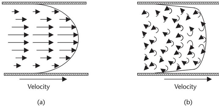
**Figure 9.1** Flow velocity variations across a pipe with (a) laminar flow, and (b) turbulent flow.
