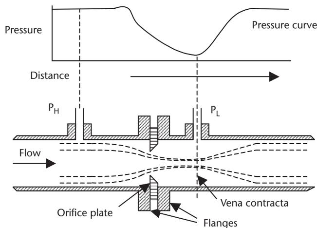
Figure 9.5 Orifice constriction plate with pressure profile.
