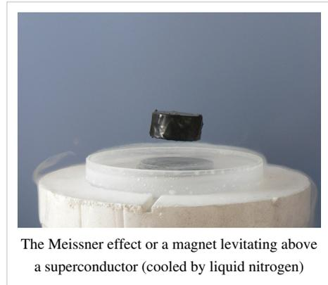
The Meissner effect or a magnet levitating above a superconductor (cooled by liquid nitrogen)
