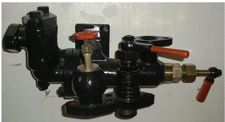
Steam injector of a steam locomotive boiler.
