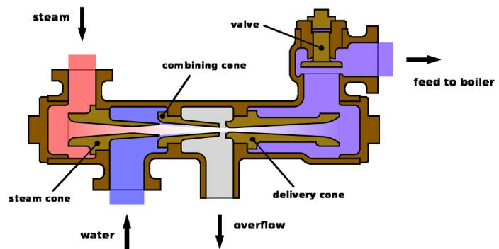
A more modern drawing of the injector used in steam locomotives.
